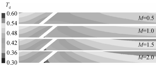
图 20 有复合角平板的子午面的温度云图 (沿 Y 方向看, \alpha=30^\circ, \beta=45^\circ ) Fig. 20 Temperature contours on meridian section of flat-plate with compound angle (view in the Y-direction, \alpha=30^\circ, \beta=45^\circ )
